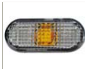
Side Blinker Unit 18-3585-01-2 RH=LH White (E13) 08/1995-09/1997, with amber inner lens
