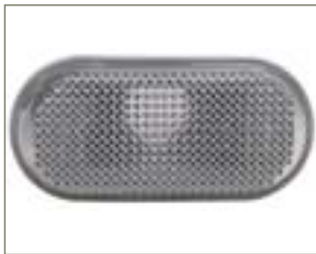
Side Blinker Unit 18-0529-01-2 RH=LH White 26160-AX00A / 26160-AX001 (E13)
